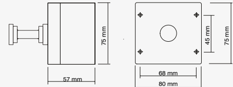
Simple Apparatus GRP junction box with nylon grounding clamp stowage pin
